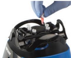
0.5 mL microfuge tubes x 6 (vertically mounted)
