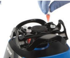
1.5/2.0 mL microfuge tubes x 4 (vertically mounted)
